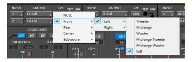
Options on the "Link" are for combine setting for Left CH and Right CH . Options on the Left CH/right CH allow you tone each selected channel respectively.
