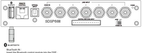
Insert the Bluetooth control module into the DSP. turn on your mobile phone and find the Bluetooth control mode. Click on the Bluetooth. When the control module is automatically Paired successful. Then you can play the music and main volume control. DO NOT INSERT THE USB.
