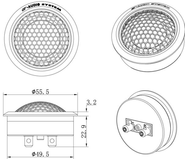
Recommended Frequency Cut: high pass up to 1500Hz
